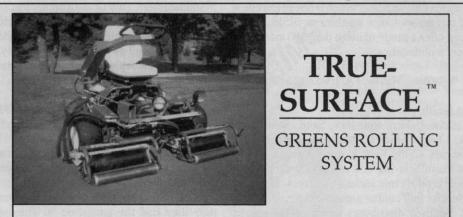
The new TRUE-SURFACE<sup>™</sup> vibratory rolling system uses an unbalanced center shaft with an eccentric flyweight to create needed movement of the outer roller, resulting in a smoother and faster putting surface. The "Quick Attach" system allows installation on most riding greens mowers in minutes.
