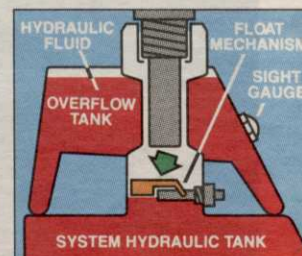
When oil leaks, fluid level drops, lowering float mechanism and setting off the alarm.
