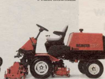
REELMASTER 335-D 2 wheel drive, diesel powered 7 blade floating head.
