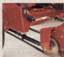
The 216 offers a unique reel drive system that maintains constant belt tension.
