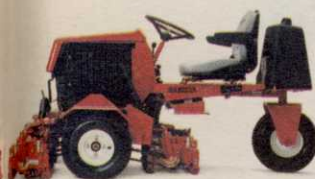
REELMASTER 216-D 2 wheel drive, diesel powered 11 blade floating head.
