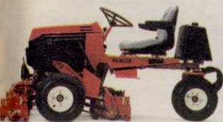
REELMASTER 216 3 wheel drive, gasoline powered 11 blade floating head.
