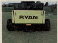
supplemental aerator with adjustable depths up to 3" and variable spacing on the GA30. The kits include holders and 1/4" solid tines which easily mount in just minutes. There's no mess to clean up after aeration. No hoses to drag around. No high price to justify.
