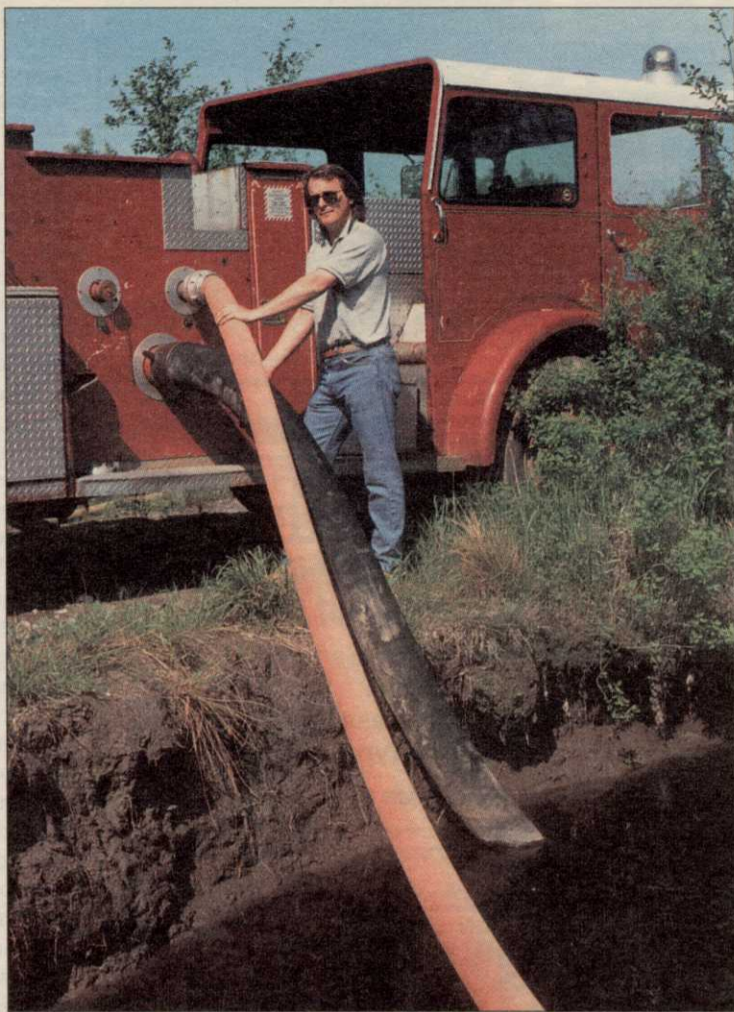
Superintendent and owner Joey Golden, left, hooks up the 1963 American LaFrance fire truck that pumps water to the entire 200-acre Springbrook Golf Club course in Leeds, Maine. The 1946 Buffalo, above, which preceded the LaFrance, rests nearby.
