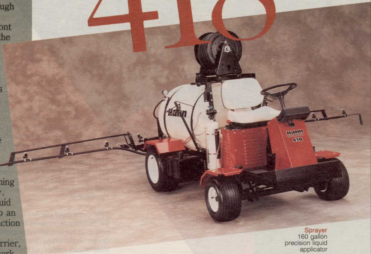
Go Boom! Independent electric controls raise and lower boom extensions
