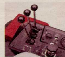
The 335 offers independent reel control levers and variable reel speed control knob.
