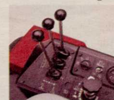
The 335 offers independent reel control levers and variable reel speed control knob.
