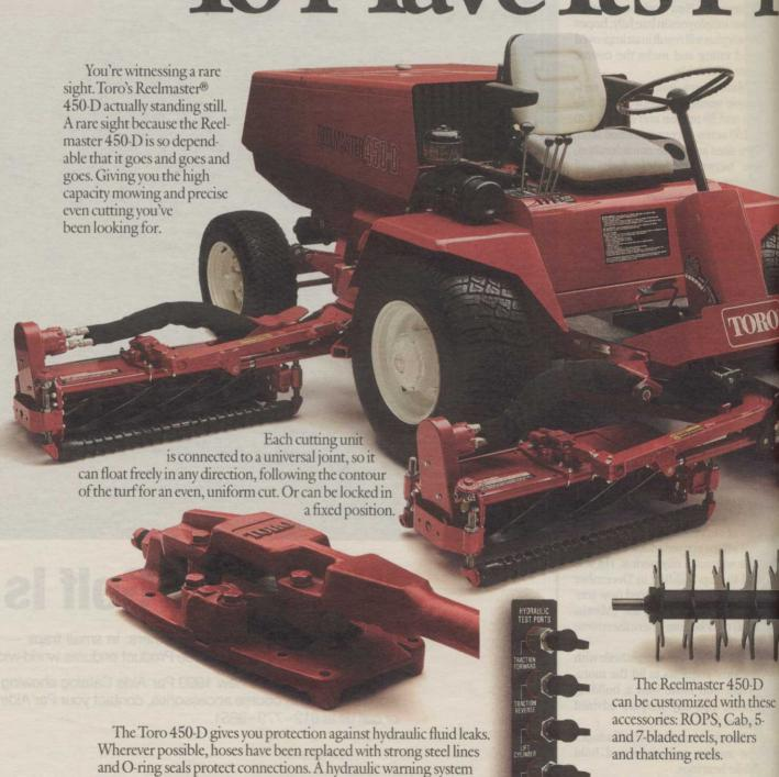
flashes an alarm when the fluid level drops. For easy servicing, test
