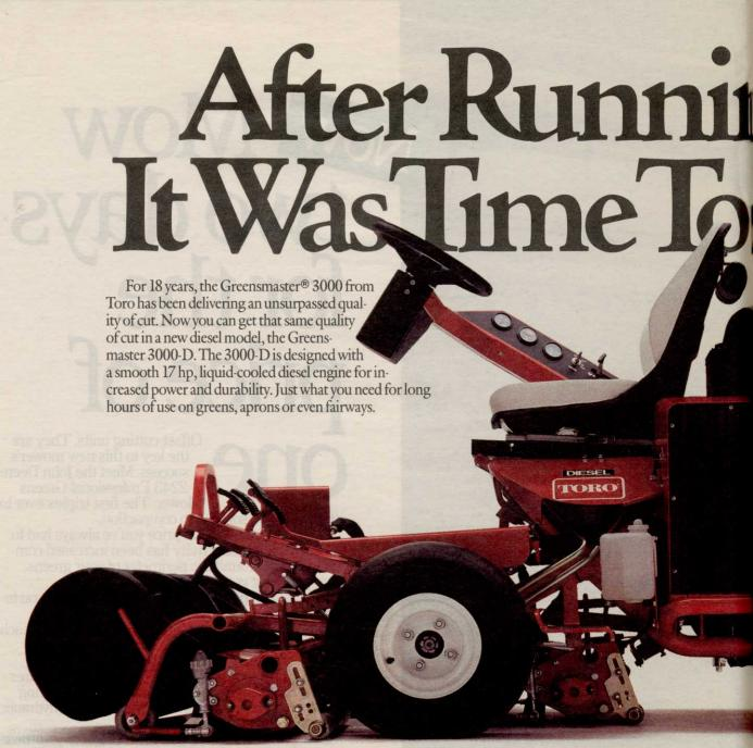
Toro's 5, 8 and 11 bladed cutting units in combination with an optional variable speed kit help make this precision cutting possible by allowing you to select a consistent ground speed while maintaining a constant, even clip.
