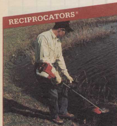
RECIPROCATORS® The RedMax Reciprocator's® two multi-tooth blades move in a scissor-like motion to more easily and safely edge, prune, hedge and trim along flower beds, around sand traps, in trees and under water.
