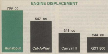
The proven, Cushman 222 overhead valve engine provides greater displacement for more torque and horsepower in the critical RPM range required for turf applications. A beefier, boxedchannel frame of carbon steel accommodates heavier implements and a one-ton payload.
