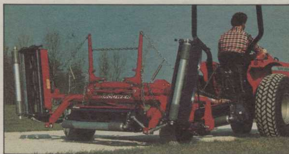
2. Hydraulic lift for easy transport or storage
