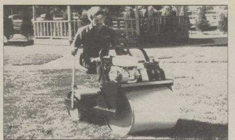
Both models are powered by a 5horsepower Honda gas engine and hydrostatic drive. The Riding Rollaire has a clutchless twin planetary transmission with a single-lever shift for forward and reverse. Write Sales Department, Cushman Division, P.O. Box 82409, Lincoln, Neb. 68501; (800) 228-4444. Circle No 350
