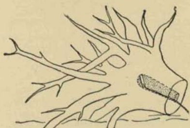
FIG. 6. SHOWING LOCATION OF A CHARGE OF EXPLOSIVES IN A HOLLOW-PULLED STUMP.
