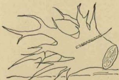
FIG. 7. LOCATION OF A HOLE BORED INTO A PULLED STUMP FOR SPLITTING. SOME PREFER TO BORE SUCH A HOLE IN THE SAME DIRECTION AS THE NATURAL HOLLOW (FIG. 6).
