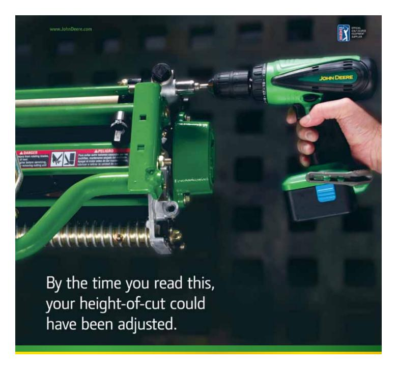
**New Quick Adjust Reels.** Yes it's now this easy to adjust the height-of-cut. Just click in a power drill on either side of the cutting unit, hit the trigger, watch the gauge, and you're done. No wrenches, and no need to double-check both sides. Thanks to SpeedLink technology, they match perfectly every time. But don't just read about these reels. See them for yourself. Call your John Deere Golf distributor for a demo. **Consider us part of your crew.**
