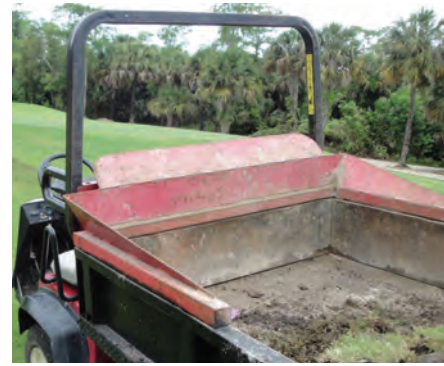
Custom-made rack prevents loads from shifting forward causing injury or damage. Photo by Darren Davis.
