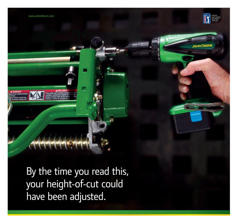
**New Quick Adjust Reels.** Yes it's now this easy to adjust the height-of-cut. Just click in a power drill on either side of the cutting unit, hit the trigger, watch the gauge, and you're done. No wrenches, and no need to double-check both sides. Thanks to SpeedLink technology, they match perfectly every time. But don't just read about these reels. See them for yourself. Call your John Deere Golf distributor for a demo. **Consider us part of your crew.**
