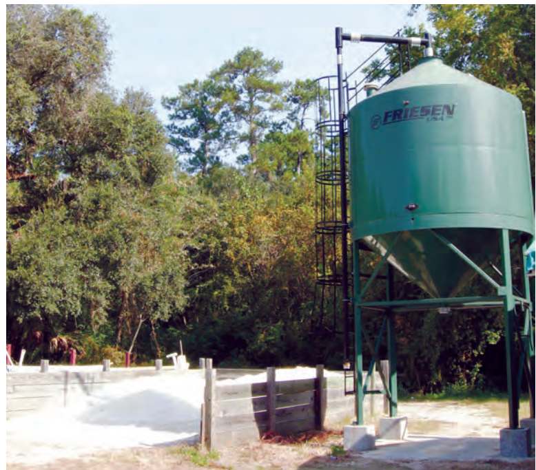
The new sand silo, above, holds dry topdressing stands beside a traditional open sand storage bin. Photo by Joel Jackson
