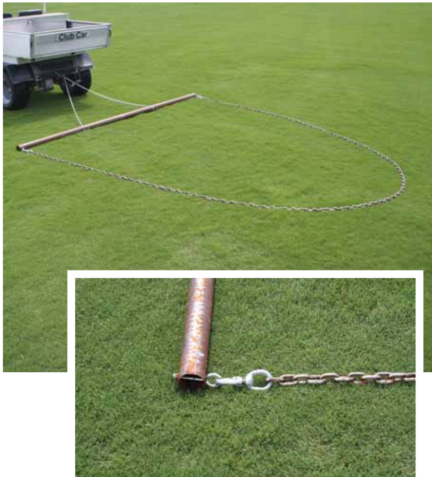
Top: This heavy-duty, yet simple-to-construct, drag not only eliminates dew for special early morning events it also busts up aerification cores during renovation. Photo by Darren Davis
