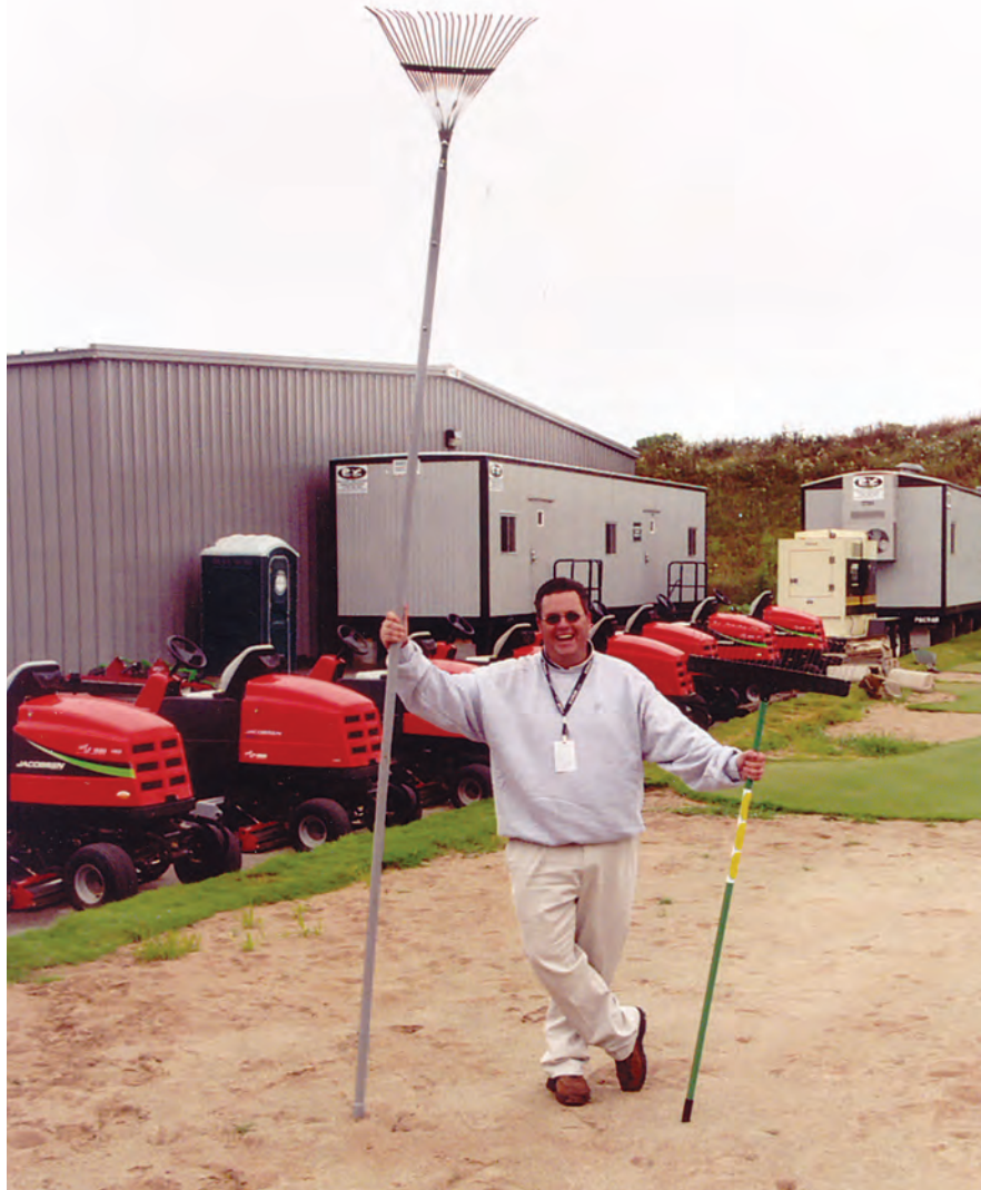
Whistling Straits Superintendent David Swift shows a standard bunker rake and one of the long-handled hybrids he developed to maintain the bunkers. Photo by Darren Davis.
