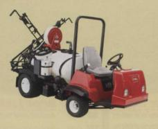
Toro<sup>®</sup> Multi Pro<sup>®</sup> 1200 and 1250 sprayers: Featuring the innovative Spray Pro<sup>™</sup> control system that directly links flow rate to ground speed ensuring precise application rate. Who to better understand a perfectionist than a perfectionist.
