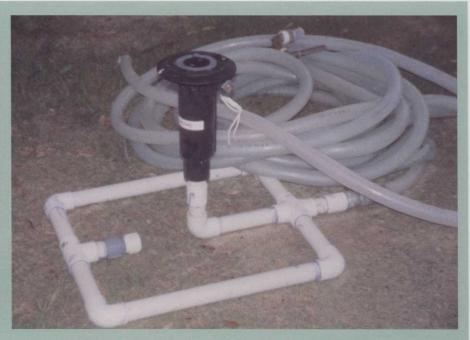
Easy and affordable to construct, this portable 1-1/2-inch PVC base is stable and delivers extra irrigation where needed at optimum pressure. Photo by Darren Davis.
