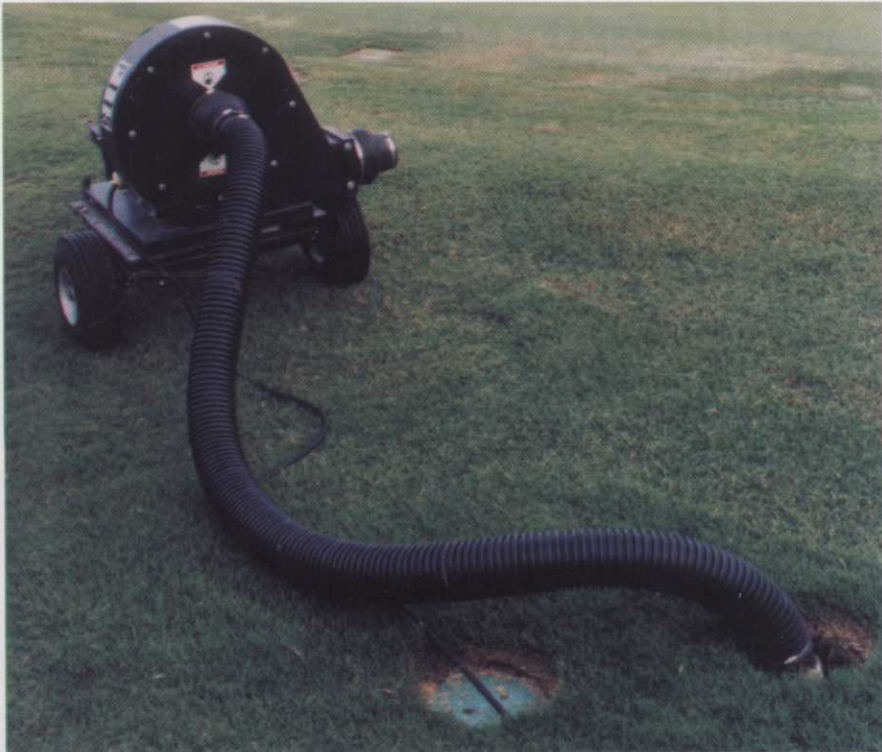
Quail West has several portable air handlers like this one that can be hooked up to each green's drainage system to move air through the root zone. Photo by Joel Jackson.
