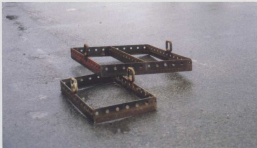
Bigger than standard pluggers. Less damaging than a sod cutter: Welded bedknives with lifting rings surgically remove Paspalum off-type patches in TifEagle greens. Photo by Darren Davis.
