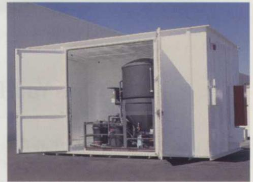
*The Turnkey Washwater Treatment System is an above ground, closed-loop, self-contained unit with zero discharge*
