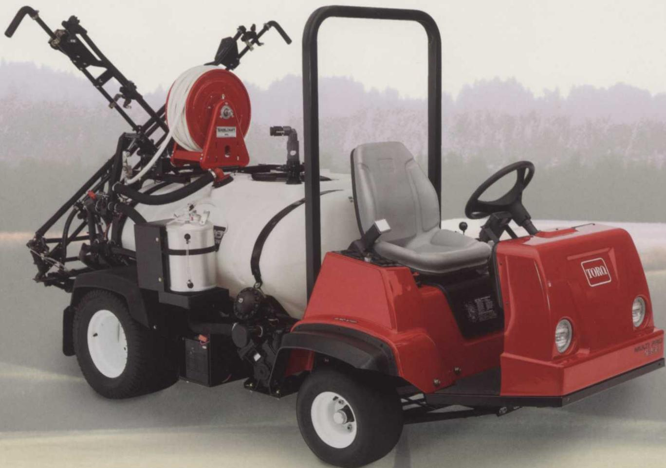
**1200** This rugged, economical performer utilizes a manual spray control system with levers to control boom spray on/off and a dial for flow rate adjustment. Includes the Spray Pro system.
