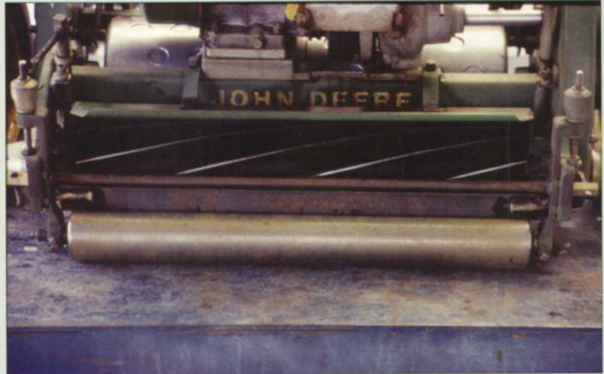
Front view of roller scraper mounted on walking greens mower. Photo by Darren Davis.
