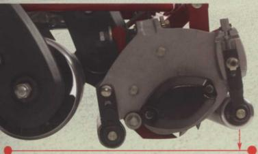
The cutting unit sets down softly back roller first, then front, like an airplane landing, to prevent gouging.
