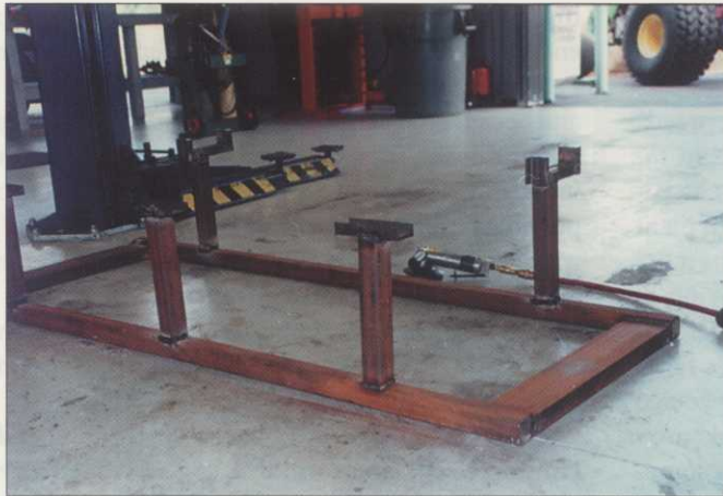
Note the three rear risers with the parallel C channel cradles and the two front risers with the perpendicular cradles. Photo by Darren Davis.
