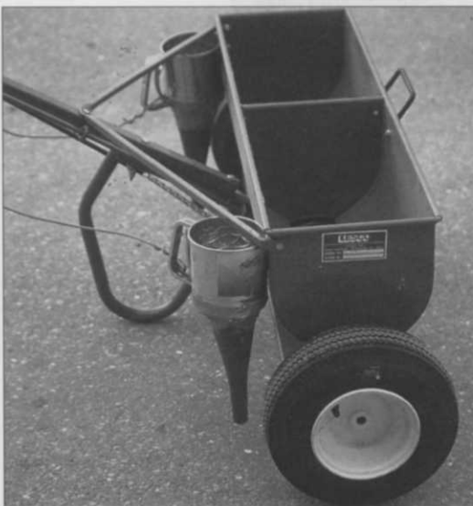
Side view of spreader shows the control cord connection to the dispenser’s triggers. Photo by Darren Davis.
