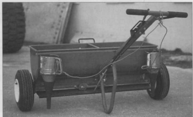
Rear view of the spreader shows positioning of the flour dispensers at the edge of the seed drop line. Photo by Darren Davis.
