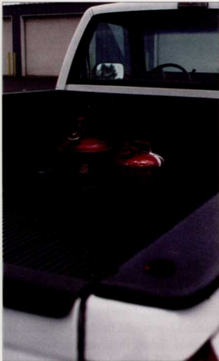
Gas cans and plastic bed liners make for a potentially dangerous combination. Photo by Joel Jackson.
