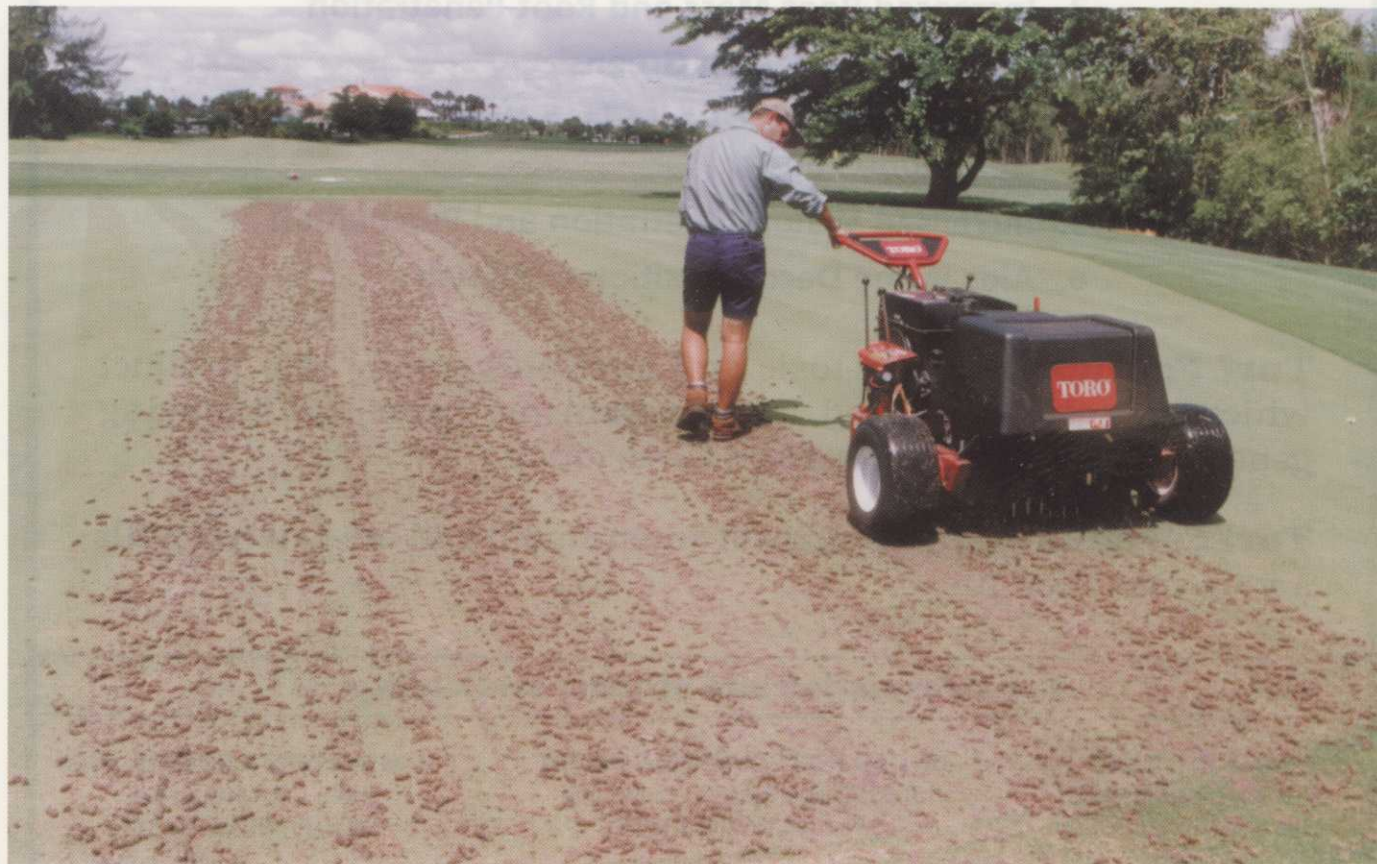
Make sure that slicing and verticutting blades are straight with good bearings. Aerifiers should be properly timed so the tines enter and exit the soil cleanly.
