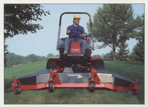
landscape and industrial grounds. Groundsmaster® 455-D efficiently mows at 6.5 mph (up to 8 acres per hour) and quickly transports from site to site at 15 mph. And it maneuvers through or transports within a 75" opening.
