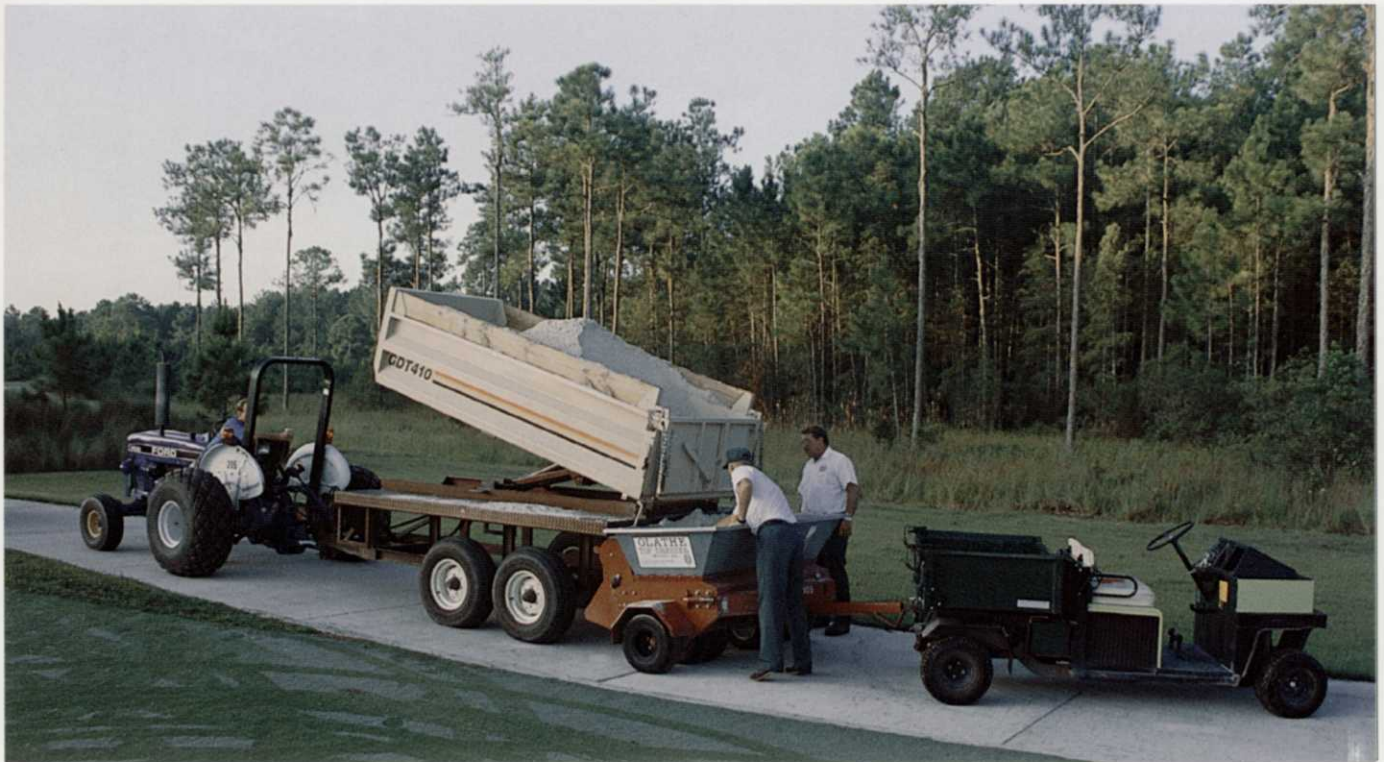
Bill King (left) and Eagle Pines working foreman, Bill Manson (right), use a modified dump trailer to refill the spreader at each green.
