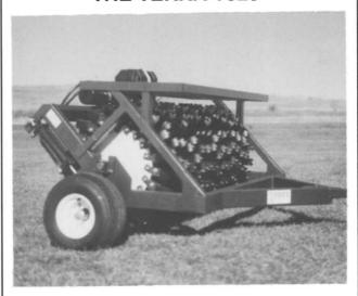
Get the job done before the golfer knows you've started. Designed for fairways and large turf areas, the Terra 320 can aerate 3 acres per hour with 3 1/2" X 4" hole spacing. High production combined with low maintenance and initial cost make it the cheapest way by far to put holes in the ground.
