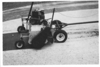
For brushing in topdressing or windrowing aerating cores: Do it with the Terra Soft Tender Rotary Broom.
