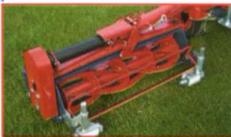
Fixed cutting unit, with anti-scalp rollers.
