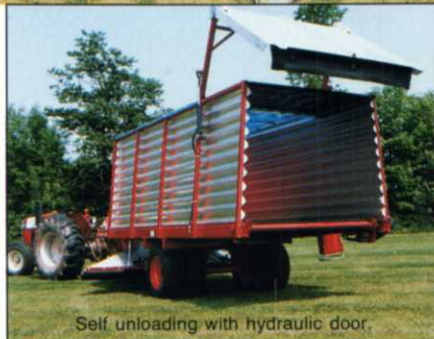
Self unloading with hydraulic door.
