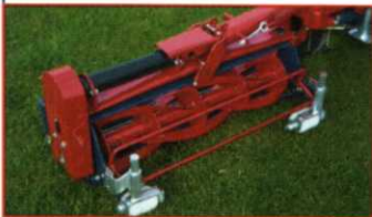
Fixed cutting unit, with anti-scalp rollers.
