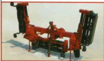
Rear mower assembly detached
