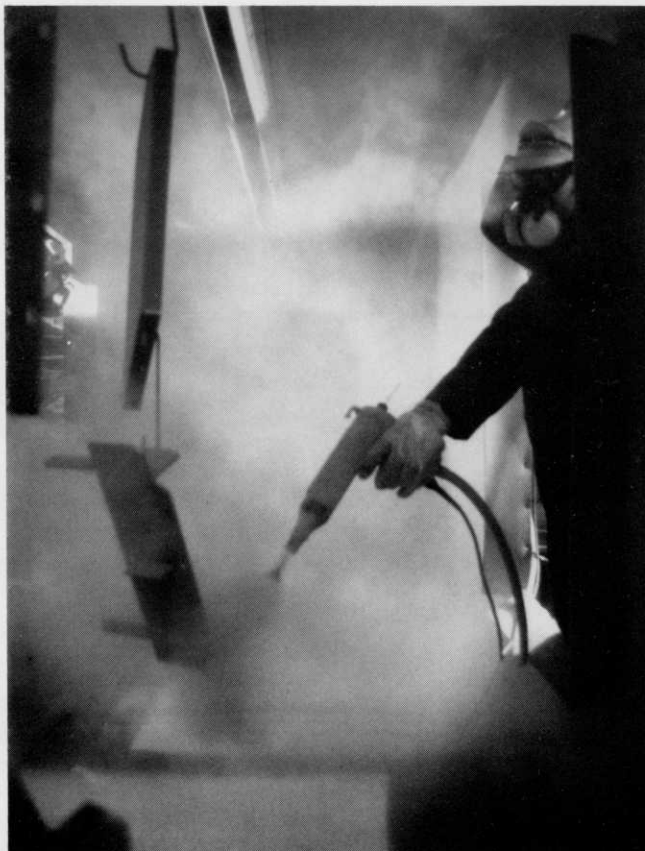
Powder Paint is electrostatically sprayed, then oven baked to a shiny gloss.
