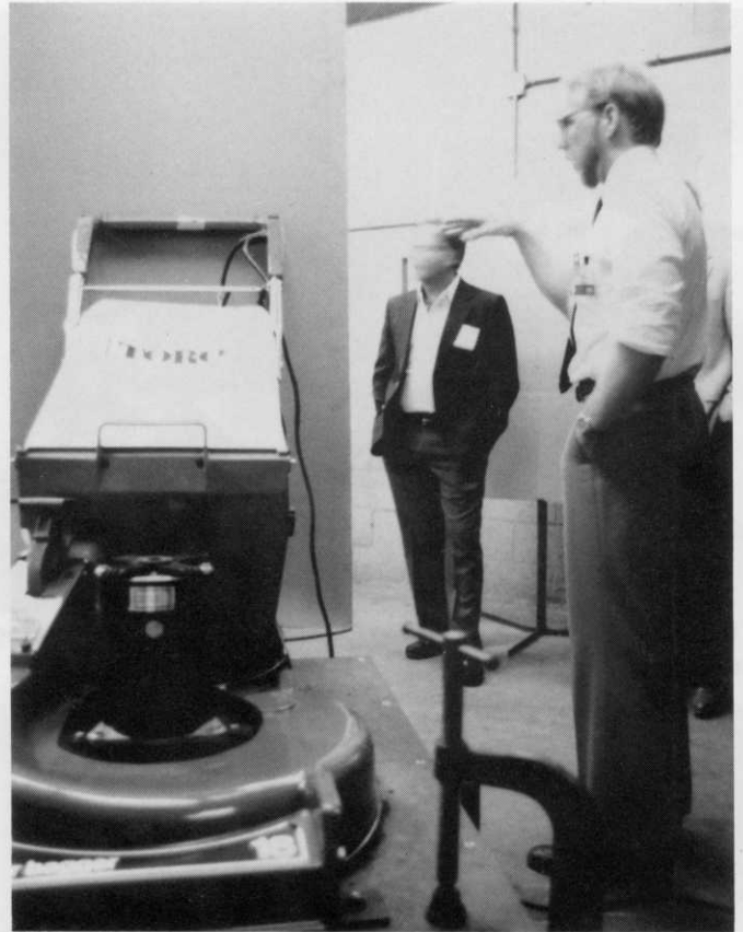
Metalavings are injected into a whirling blade for shatter testing.
