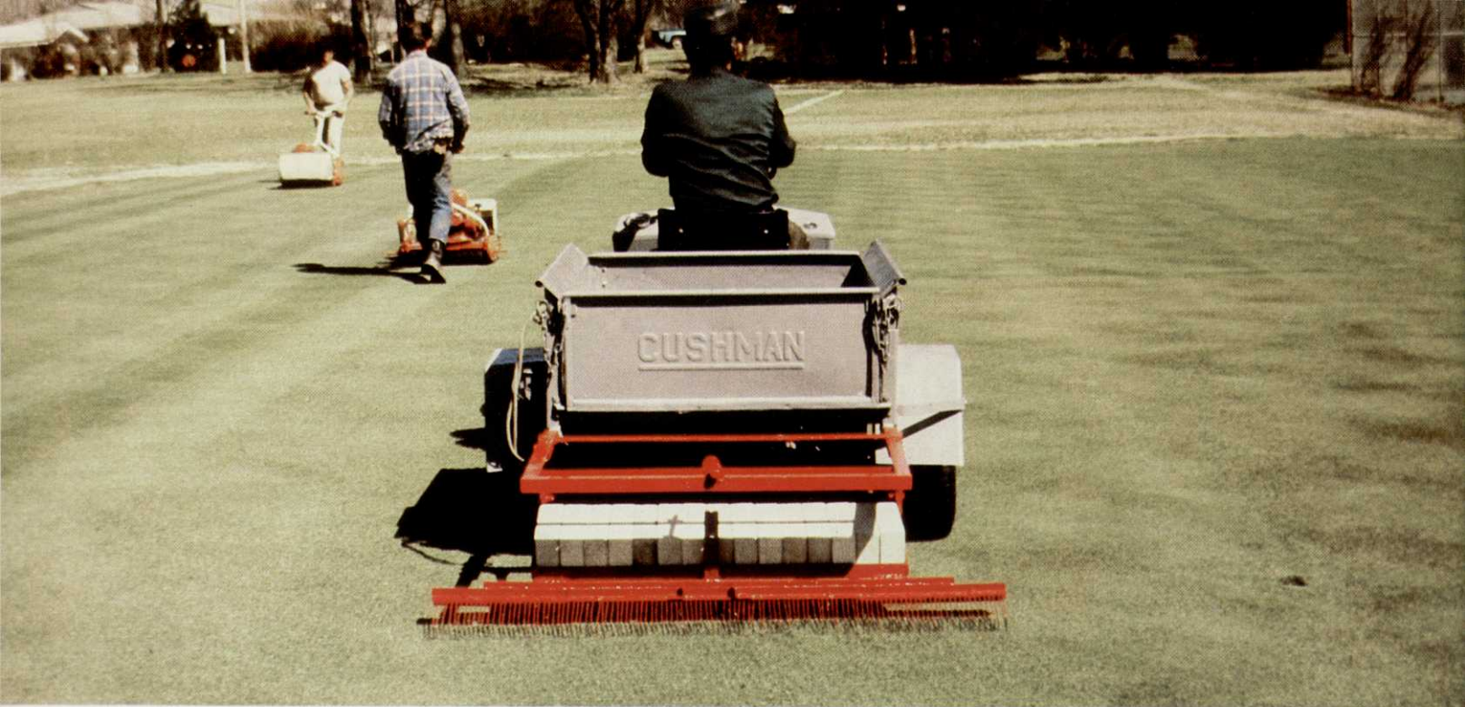
(Above) Delmonte rake removing excessive thatch from a green. Heavy thatch affects green speed and putting consistency.
