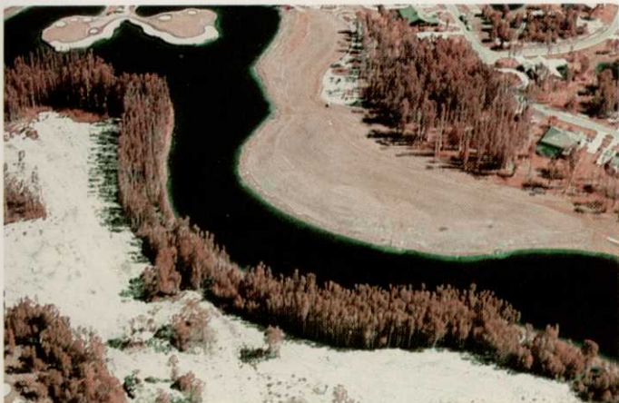
The two dark spots, immediately forward and to the left of the tee at Fiddlesticks in Ft. Myers, are subsurface leaks in the irrigation line. Not detectable from the surface.
