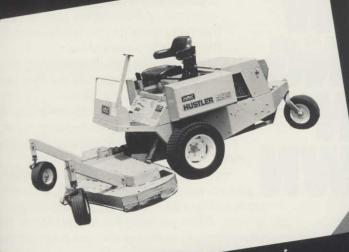
THE EXCEL HUSTLER is the most maneuverable of all out-front riding rotaries. It features a dual hydrostatic system that directs INFINITELY VARIABLE speed, direction, and braking through each drive wheel; all operated by one convenient hand control.
