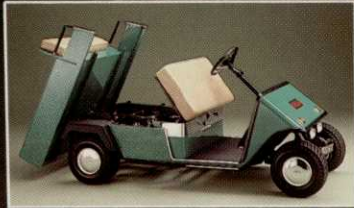
The load bed tilts for easy access to the drive package.
