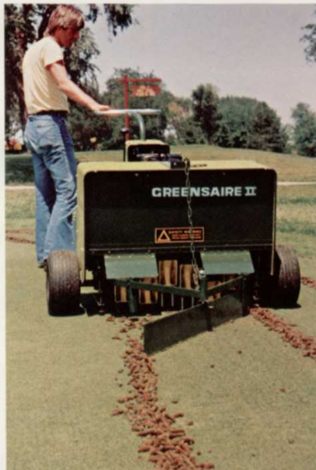
Greensaire II with optional windrow attachment.
