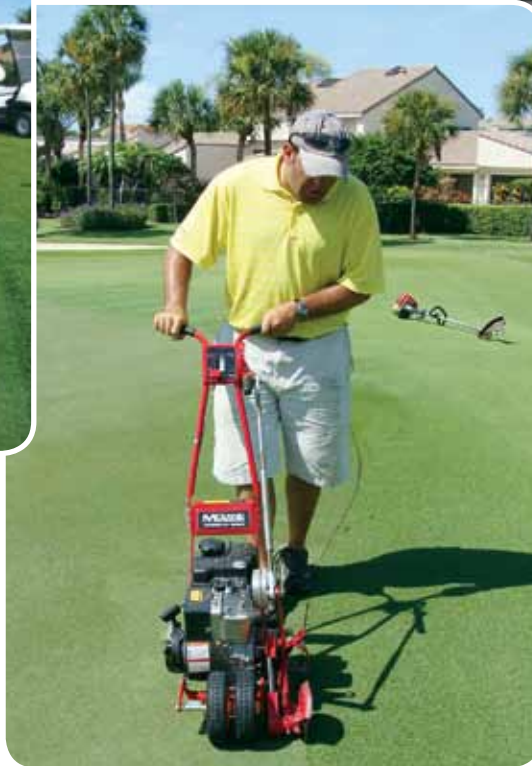
Stick edgers like the one above are commonly used to define the edge of the putting surface. Some workers prefer the McCune edger on the left for more control. Photos by Jim Sprankle, CGCS (above) and Steve Wright, CGCS (left).
