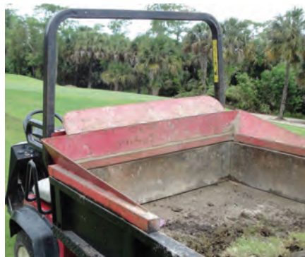
Custom-made rack prevents loads from shifting forward causing injury or damage. Photo by Darren Davis.
