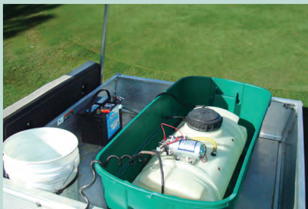
A 50-gallon storage container eliminates the risk of leaks from portable sprayers. Photo by Darren Davis.
