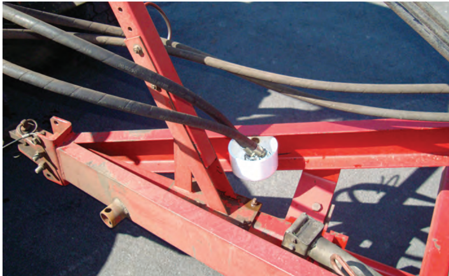
Placing disconnected hydraulic hoses in this handy hose cup prevents spills and slip hazards. Photo by Darren Davis.
