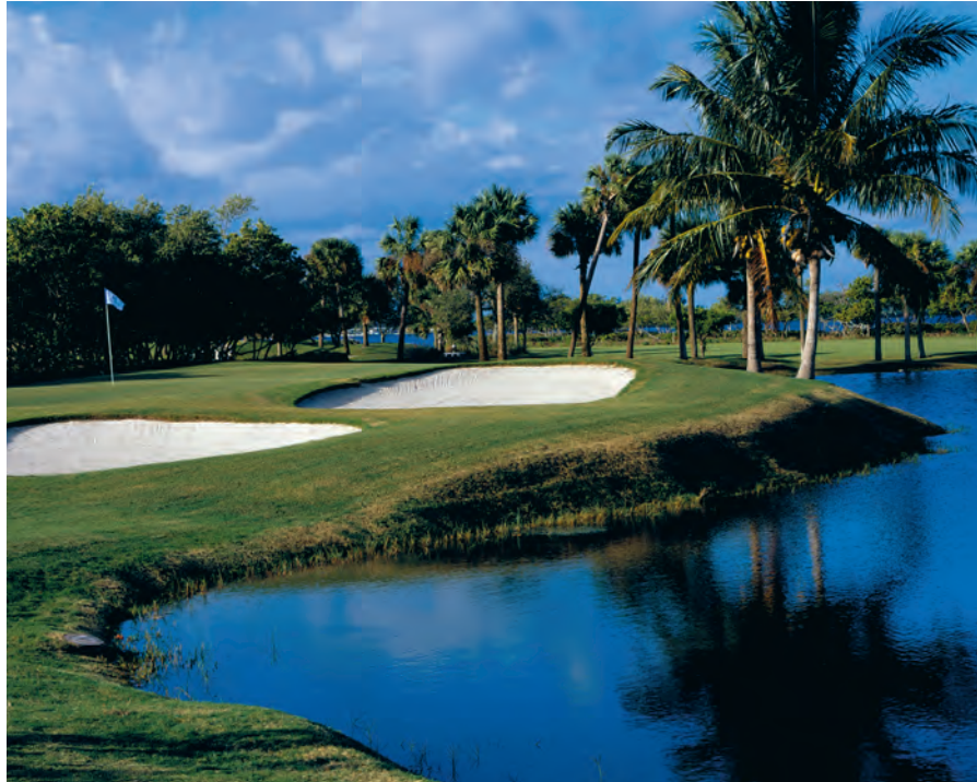
This lake guarding the par 3, 9th hole is part of a nine-lake, 5-acre network which stores stormwater and provides back up irrigation. Photo by Daniel Zelazek.
