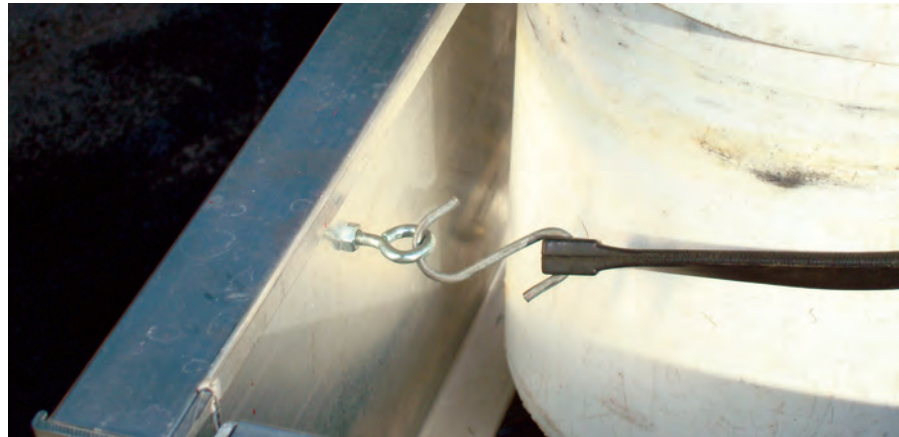
Two 1/4-inch eye bolts and a 21-inch strap with an S-hook secure the bucket. Photo by Darren Davis.
