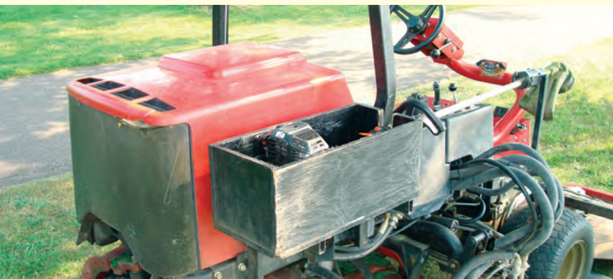
At the famed Hazeltine Golf Club in Minnesota they mount string trimmers on the trim mowers for increased productivity and operator safety. Photo by Darren Davis.
