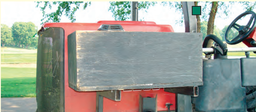
Close up of the plywood box and bracket attachment housing the motor part of the string trimmer. Photo by Darren Davis.
