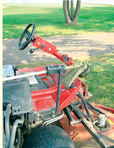
Close up of the PVC section and bracket that holds the string trimmer shaft. Photo
