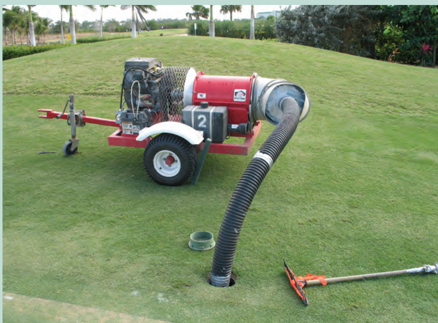
A fairway blower can be used as a portable subsurface air pump for problem greens. Photo by Mark Jacobs
